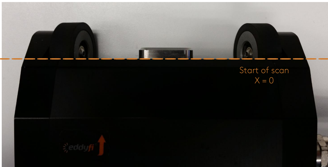
Figure 93. Scan position x=0 aligned with the front of the probe
