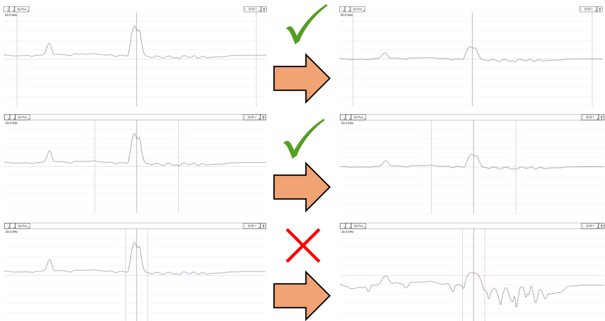
Figure 82 : Top : Good user material calibration, with the C-scan cursor widely opened; Middle : Good user material calibration, cursor contains only one specific crack, but opened wide enough (at least three times the length of the crack) providing a local averaging; Bottom : Bad user material calibration, cursor too closed around the crack signal. The user material is not well measured because there is not enough safe material information in it, averaging mostly calculated on the crack signal.
