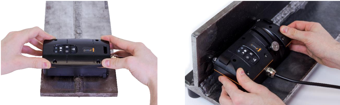
Figure 50. Sharck probes on carbon steel weld
